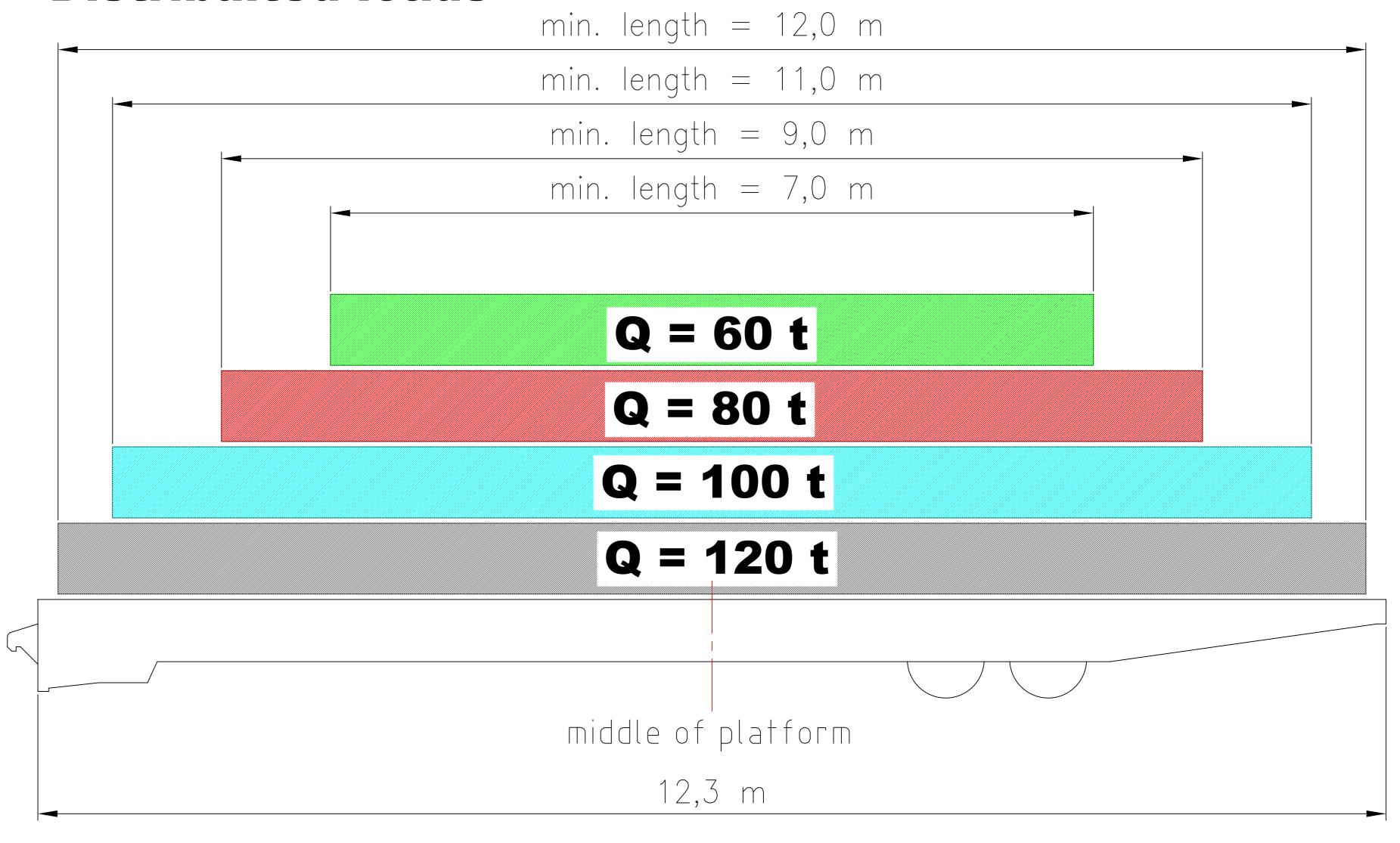
Load gravity center must be inside the rispective marked areas
